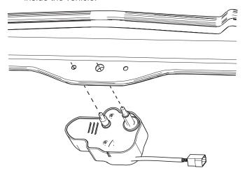
4. Fit a small rubber washer and a small cupped washer over the mounting stud then fasten the stud nut to the mounting stud to hold the motor in place.
