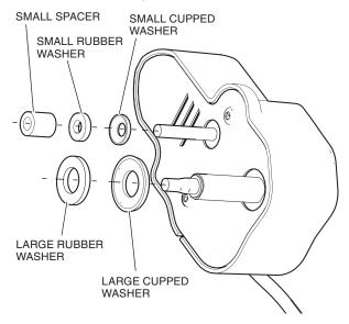
Insert the motor into the windshield so the motor spindle fits through the center hole and the mounting stud fits through the right most hole as viewed from inside the vehicle.
