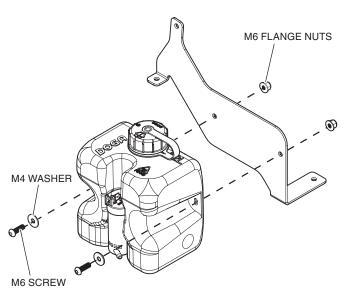
Position the washer tank and bracket inside the front of the vehicle so the bracket lines up with the P-clips, then fasten one screw attaching the bracket to the vehicle frame.
