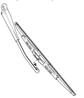
9. Fit the wiper arm over the motor spindle parallel to the top left side of the windshield.
