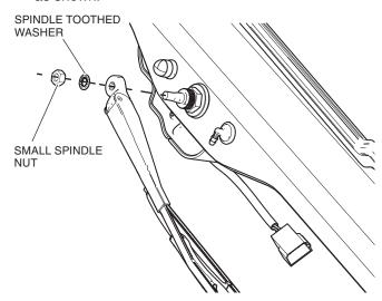
11. Connect the wiper hose from the wiper arm to the elbow connector.
