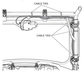
7. Run the wiring harness and washer hose into the gap in the side of the vehicle and under the hood to the fuse box.
