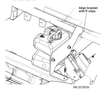
8. Attach the large P-clip to the washer tank bracket using one M6  $\times$  20 mm button head screw and one M6 flange nut as shown.
